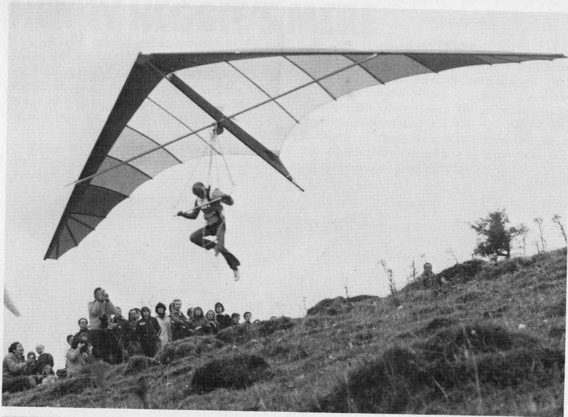
Moyes Supersoarus takes to the air showing a very flat wing section apart from an abrupt curve near the leading edge.
