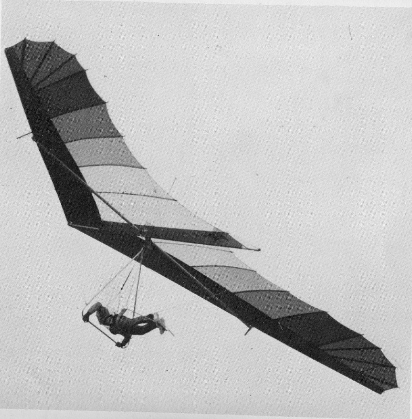
It is noticeable that Moyes uses wing wires for deflexing only and not as primary sail shapers.
